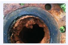
Iron and manganese often causes the main problem of the waterworks. When water gets in contacts with air, it changes the colour, turbidity increases and sediments appears. Water has a metallic taste. Water pipes are clogged and sanitation at the consumer becomes dirty. Suggested concentration of iron should be 0.1 mg/l and manganese 0.05mg/l.
