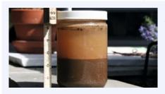
Ground water and surface water can contain sand, mud and different sediments that clog the system, wear out valves, measuring devices, etc.
