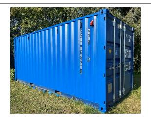
A new 20-foot sea container with dimensions: length 6.06 meters, width 2.44 meters, and height 2.40 meters. The water filtration system is placed inside the new sea container for easy transportation both by waterways and roadways.
